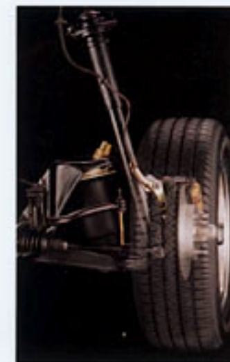
Computer-controlled air springs and nitrogen-pressurized hydraulic shock absorbers contribute to remarkable handling proficiency.
