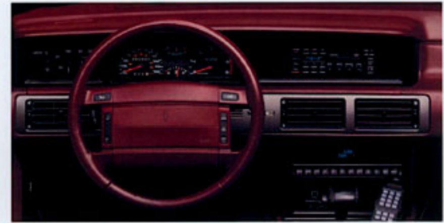
Shown here: The analog gauges of the Mark VII LSC. The Bill Blass Mark VII employs digital, electronic instrumentation.
